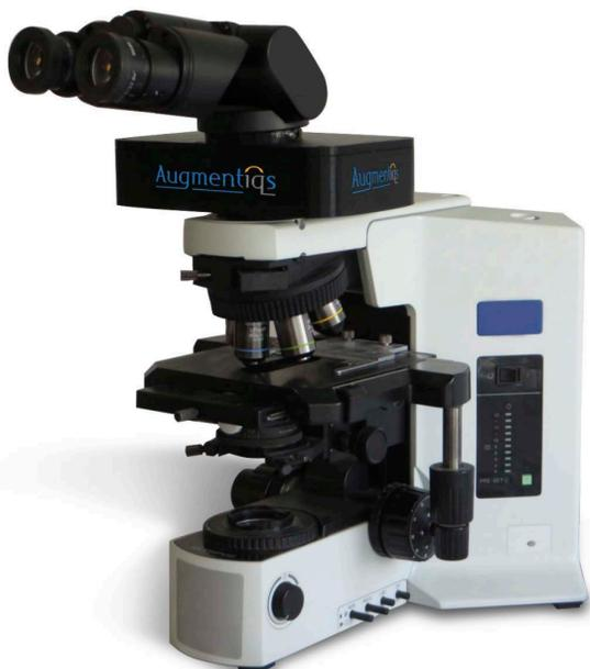
Figure 1. Optical module installed on microscope.
