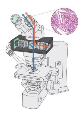
The high-resolution image capturing system obtains a Field of View (FOV) output that is close to a 1:1 view of the eyepiece (depending on the microscope and objective used). The use of a considerably efficient digital imaging sensor allows for the integration of highly sensitive software applications to be used for the enhancement of clinical efficiency.
